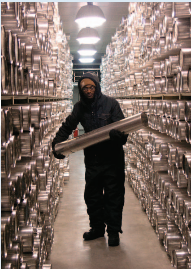
The U.S. Geological Survey National Ice Core Lab stores ice cores samples taken from polar ice caps and mountain glaciers. Ice cores provide clues about changes in Earth's climate and atmosphere going back hundreds of thousands of years.
