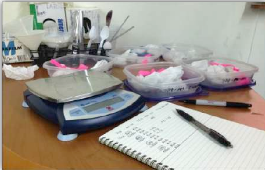
Figure 10. Outdoor Lab (top): As soon as the containers were removed from the water we drained them using coffee filters in a funnel to trap the sediments of each container at each location. Indoor Lab (bottom): The wet coffee filters were set out to dry inside the lab and once completely dry, the sediment specimens were weighed and measurements entered on paper and into excel tables.
