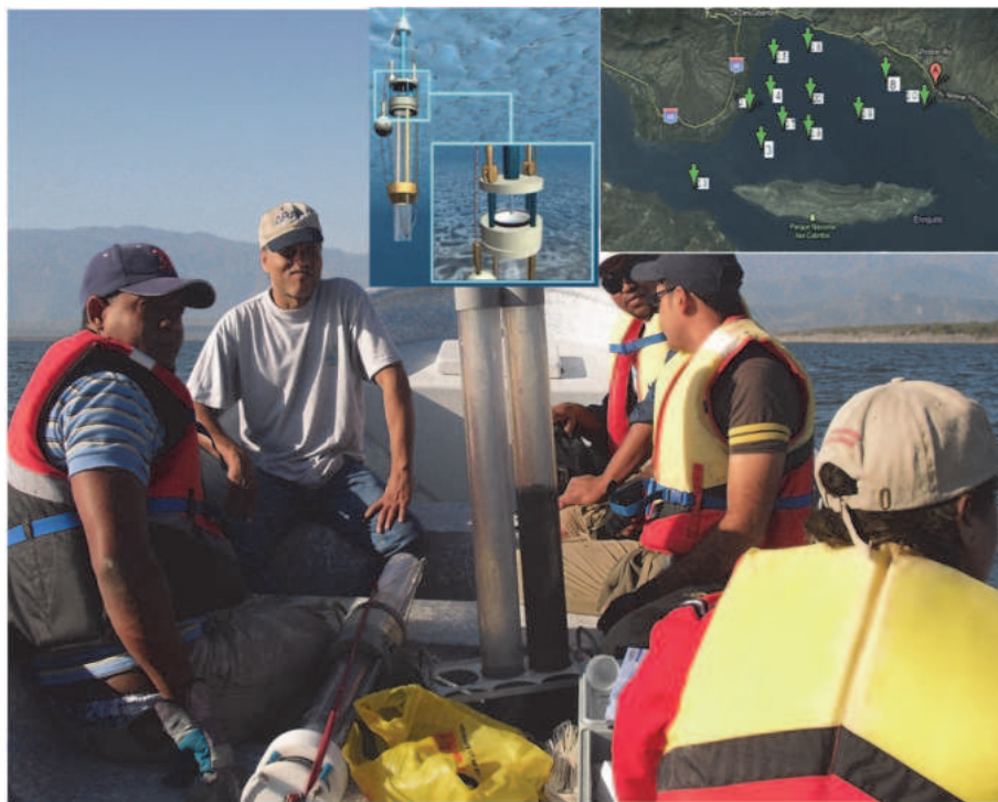
Figure 4. Sampling campaign with Uwitec sampler (horizontal position). The lengths of the tubes are 1.20 meters, the core is number 2 with a length of more than 80 cm corresponded to the zone influenced by the Los Pinos river near La Descubierta (latitude 18.5261 North and longitude 71.7311 West with a TAS = 2.55 cm a-1 (2003-2011) core number 10 (67 cm) influenced by the Guayabal River to the north, number 13 by the waters coming from Jimani and Boca de Cachón
