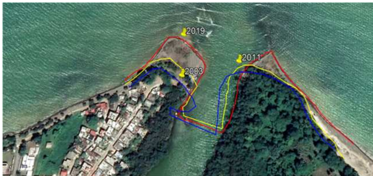
Figure 8. Mouth of the Yeguada River. The blue line represents the coastline from 2003, the yellow line from 2011, and the red line from 2019. Between 2003 and 2019, 0.01 km 2 of the bay were lost due to the entry of sediments contributed by the Yeguada River. At low tide, the river is closed to the sea by a sandbar. Source: Google Earth. Photo: Landsat 8.
