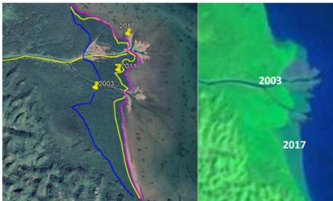
Figure 6. Mouth of the Yuna River. The blue line represents the coastline from 2003, the yellow line from 2011, and the violet line from 2017. The riverbed was always the same due to its channeling. Between 2003 and 2011, 2.00 km 2 of the bay were lost, from 2003–2017 the loss was 2.17 km 2 . All losses were caused by the entry of sediments from the Yuna River. Source: Google Earth, left; Photo: Landsat 8. https://landlook.usgs.gov/landlook/viewer.html , right.
