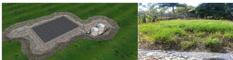
Fig. 1. “El Dorado” wetland. On the left, the conceptual plan of the treatment system and on the right, a photo of the wetland after 18 months of operation
