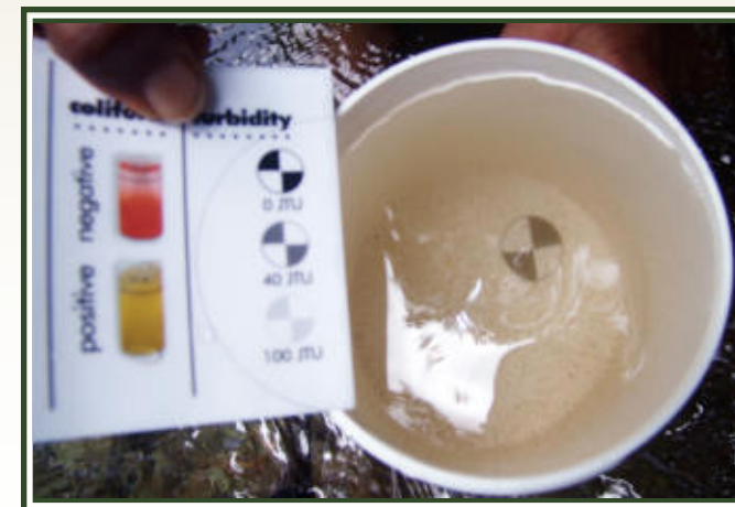
Testing for turbidity with "Green Low Cost Water Monitoring Kit"
