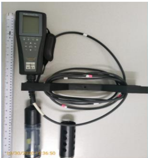
Figure 9: The YSI Multi-parameter probe which can collect the physio-chemical analysis for data collection. (Photo credits: Mona Webber)
