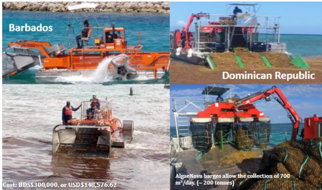
Figure 8b: The different types of Booms and Barges used in the region to handle the Sargassum influx. (Photo credits: algeanova.com and sargassumsolutionsltd.com )
