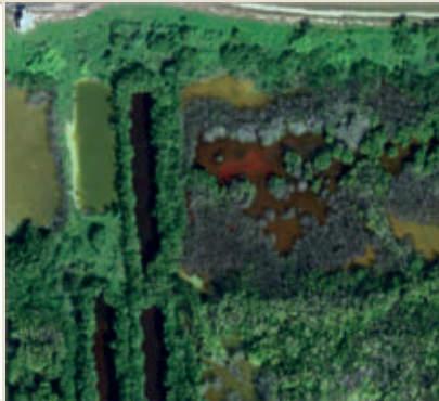
Orthomosaic generated using photogrammetric images captured with a drone camera.
