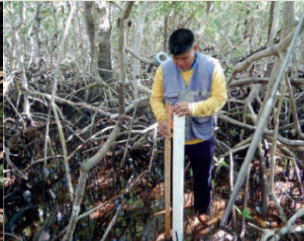
Placing automatic pressure sensor at preserved reference site
