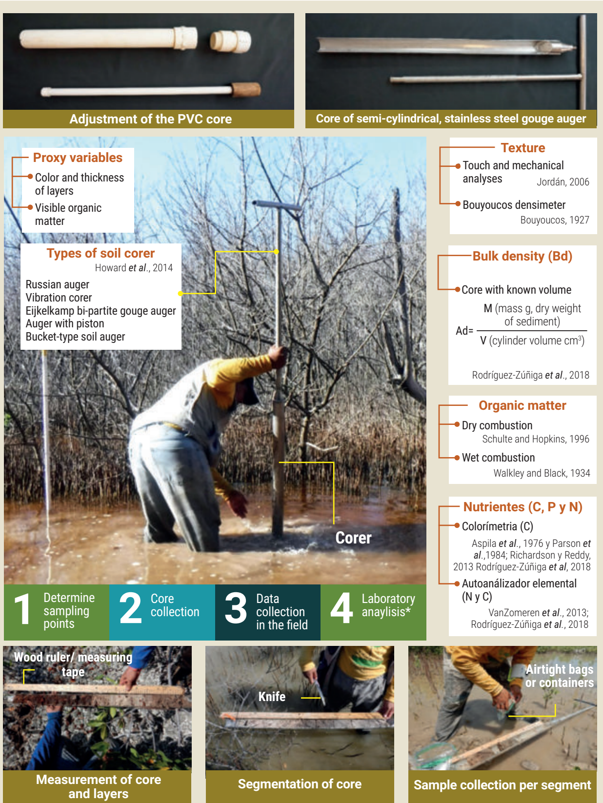
Figure 2.11 – Techniques and variables for characterizing mangrove sediment. Prepared by Oscar Pérez, Andrés Canul and Diana J. Cisneros.
