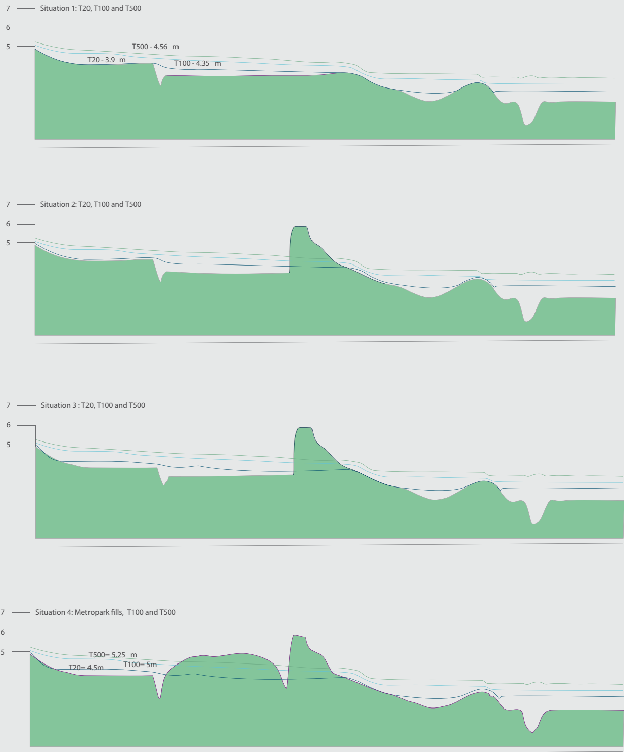
Figure 35 | Longitudinal profile showing flood levels in Situations 1-4.
